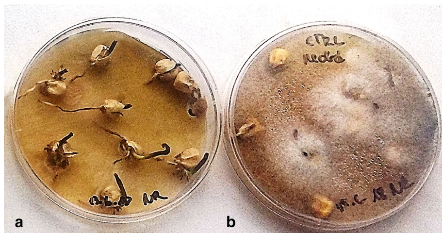
Fig. 7 Photos of a plasma-treated (3 s, 15 Pa) and b untreated (right) seeds after 7 days of incubation
