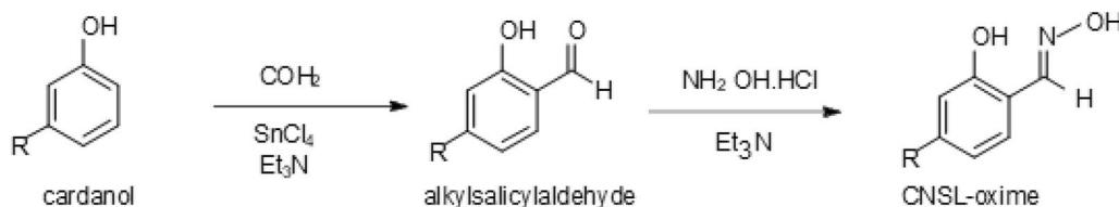
Fig. 2 Chemical reactions to produce oxime from cardanol
