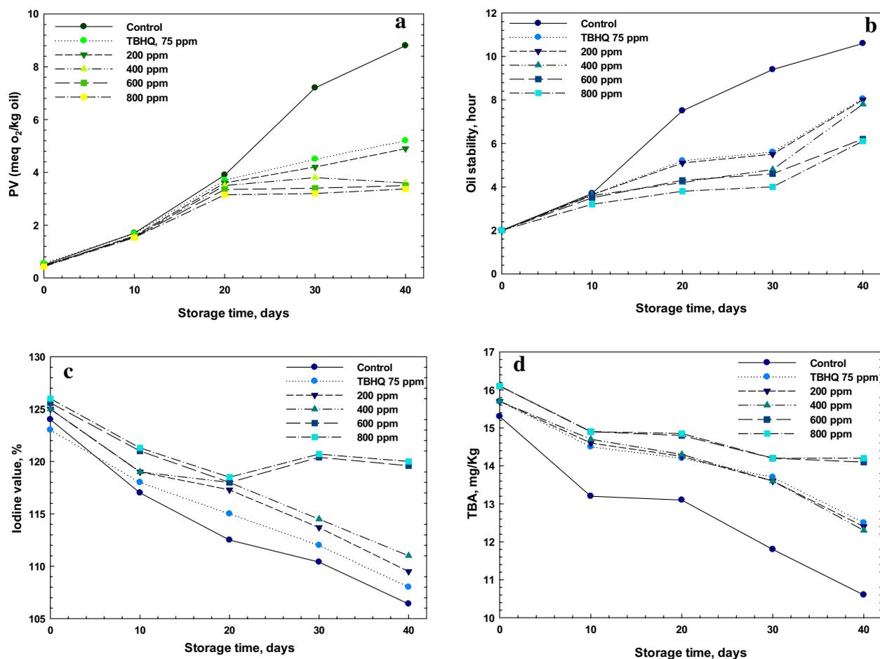
**Fig. 4** The changes of physicochemical properties of canola oil as affected by various amounts of antioxidants during storage: **a** peroxide value, **b** oil stability, **c** iodine value, and **d** TBA value
