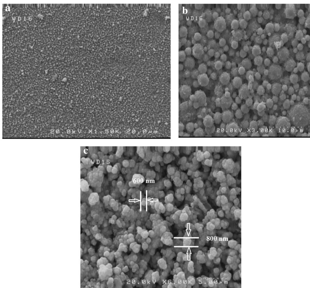
**Fig. 2** SEM micrographs of inulin (a), maltodextrin (b), and  $\beta$ -cyclodextrin (c) as wall materials in polyphenolic core
