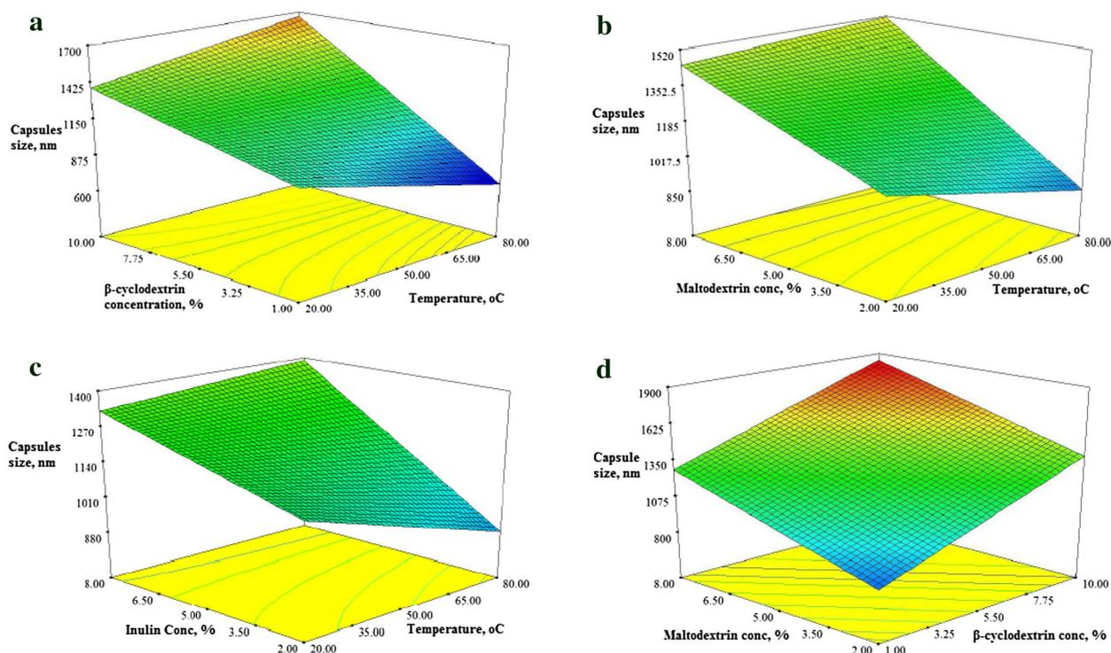
**Fig. 1** 3D graphic response-surface optimization of **a** incorporation efficiency as capsules size (nm) vs.  $\beta$ -cyclodextrin concentration (% w/w), **b** incorporation efficiency (nm) vs. maltodextrin concentration (% w/w), **c** incorporation efficiency as capsules size (nm) vs. inulin concentration (% w/w), and **d** effect of the  $\beta$ -cyclodextrin and maltodextrin concentration on the capsules size (nm)
